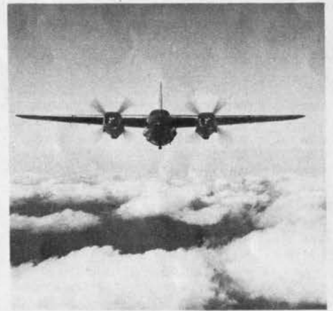
Bumps made by new guns alter the B-26's hitherto symmetrical head-on appearance.
